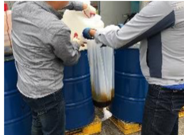
Research laboratory: solidification treatment of waste liquid
